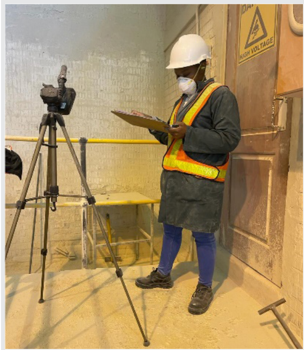
Image 12: Monitoring of respirable crystalline silica using a direct-reading instrument.
