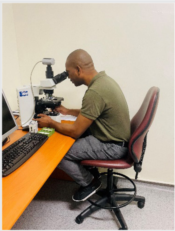
Image 10: Asbestos analysis using a Phase Contrast Microscopy in the Asbestos Laboratory.
