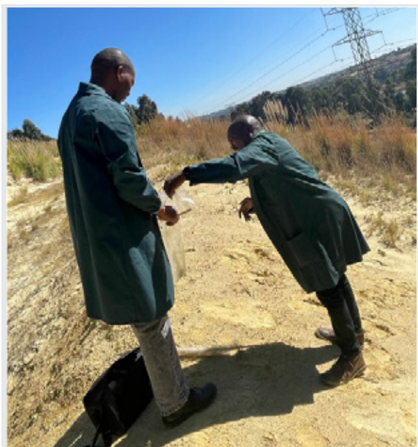
Image 13: Collecting a dust sample at a gold mine tailing dump.
